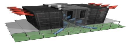
Once the aisles were enclosed, and the supply air segregated from the return air, the CRAC units could be "tuned" to deliver the correct quantity of air at a supply temperature that can safely be much closer to the desired aisle temperature. The fans do less work. The cooling system does less work and, when it is cooling, the system is
