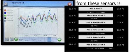
The system displays real-time temperature profiles for each of the aisles. It also records and displays trend graphs, so that performance can be readily reviewed. Data centre managers can immediately see the effects of any changes that are made to the cooling control systems (such as raising the return air set point). The aisle profiles created by the multiple sensors allows supply air registers to be "tuned" to deliver air where it will be useful rather than wasted.
